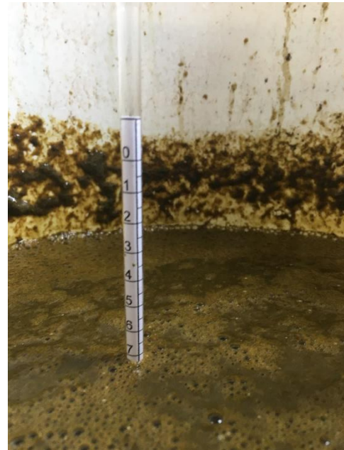
Figure 2(b): The gravity hydrometer settled in the dairy slurry sample. The measurement of 7 was
